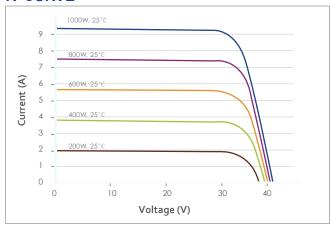
**ELECTRICAL PERFORMANCE** XS60CA-330 XS60CA-335 XS60CA-340 Electrical Performance @ STC Max. Power Voltage Vmpp(V) 33.9 34.1 34.3 Max. Power Current Impp(A) 9.74 9.83 9.92 Open Circuit Voltage Voc(V) 41.0 41.2 41.4 Short Circuit Current Isc(A) 10.33 10.38 10.44 Module Efficiency (%) 19.56% 19.85% 20.15%
